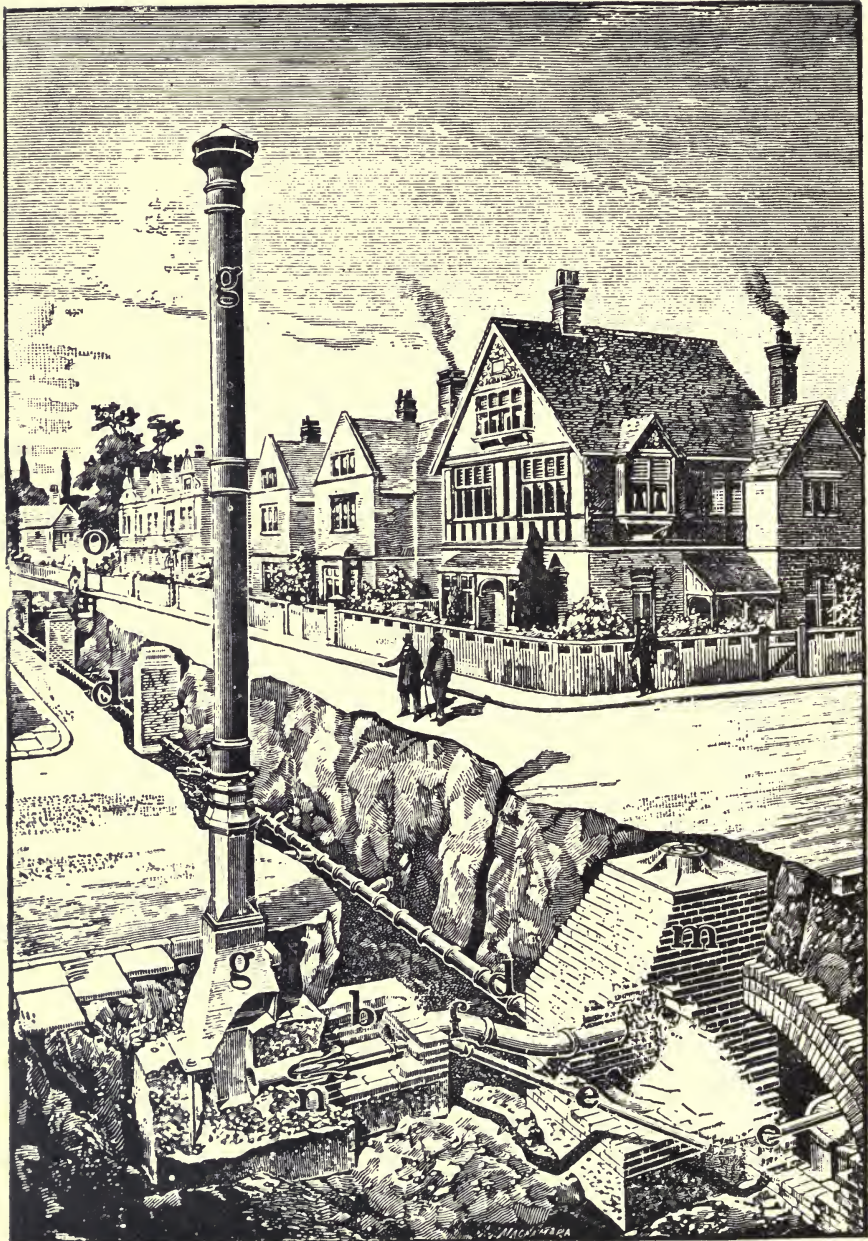
Fig. 11. Shone & Ault's Sewer Ventilating System.
